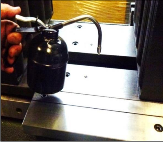
1.4) Lubricate the upper clamping blocks.
