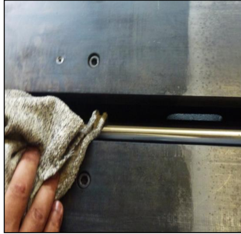
1.5) Clean the vice clamping shaft.
