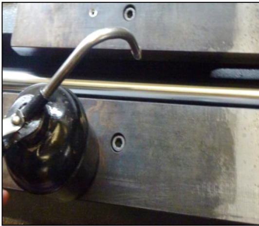
1.6) Lubricate the vice clamping shaft.
